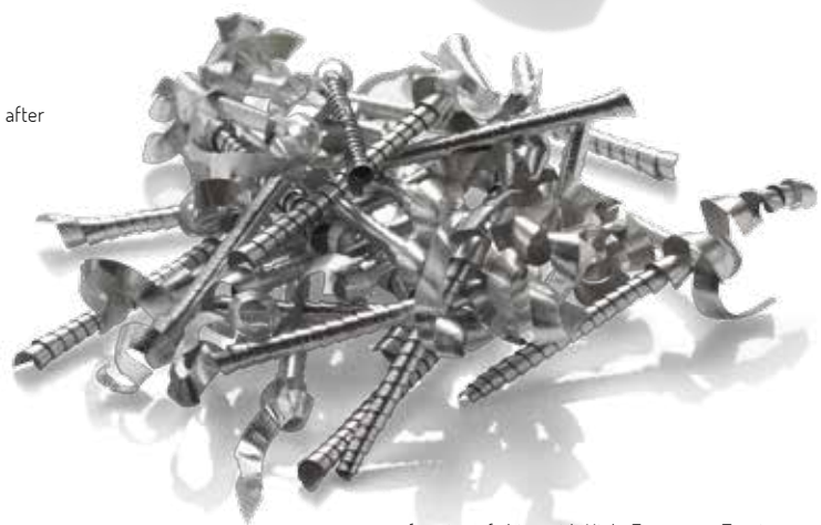
forming of chips with High-Frequency-Turning
