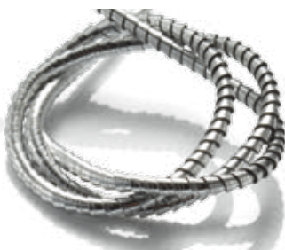
forming of chips with usual working
